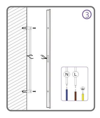
3. Connect wires to power supply (Blue for N line, brown for L line)
