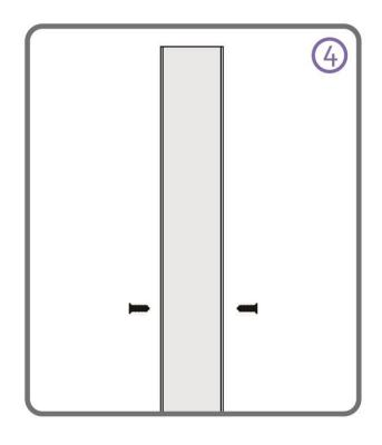
4. Attach light to mount and tighten screws
